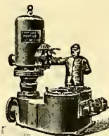
FIG. A.—This ram lifts part of the same water that works it. (Engraved from Photo. of Ram which raises 250,000 gallons per day of 24 hours to medium height, with good, working fall.)
