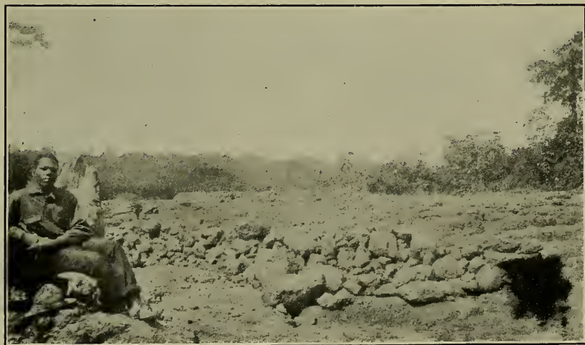
2. Bauxite at Akyma. The covering of vegetation and earth has been removed leaving the bauxite exposed. Bauxite, an oxide of aluminum, is a valuable mineral.
