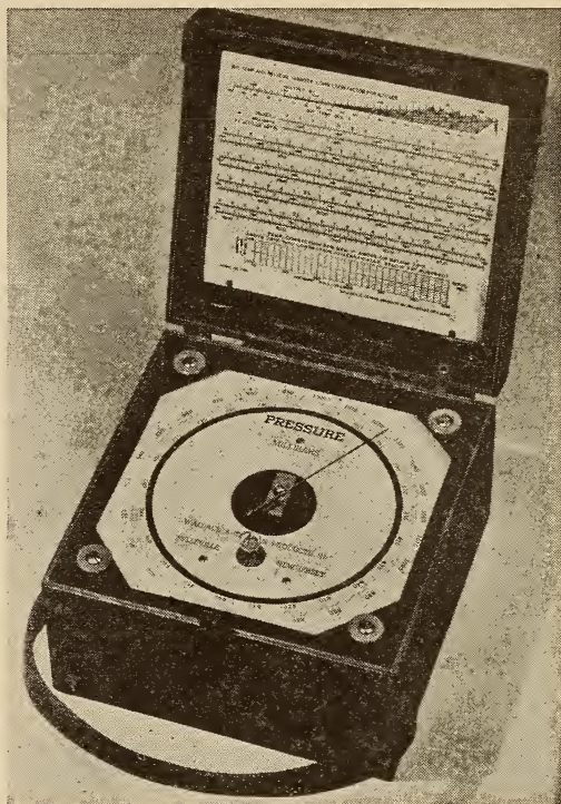
Fig. 4.—Aneroid barometer, range 610 to 1,085 millibars. Pointer makes two revolutions; scale 7\frac{1}{4} inches in diameter. The humidity and correction factor is obtained from the nomogram at the top of the cover; the conversion of pressure to altitude in the SMT standard atmosphere is given in the chart in the middle; and data on the temperature error of the barometer can be plotted on the graph at the bottom.
