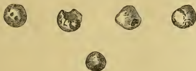
FIG. 1.—"BOMBS" PRODUCED IN THE BESSEMER PROCESS.
