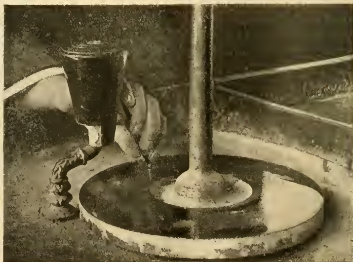
FIG. 3.—Gem held in position against the wheel. From "The Gem-Cutter's Craft."
