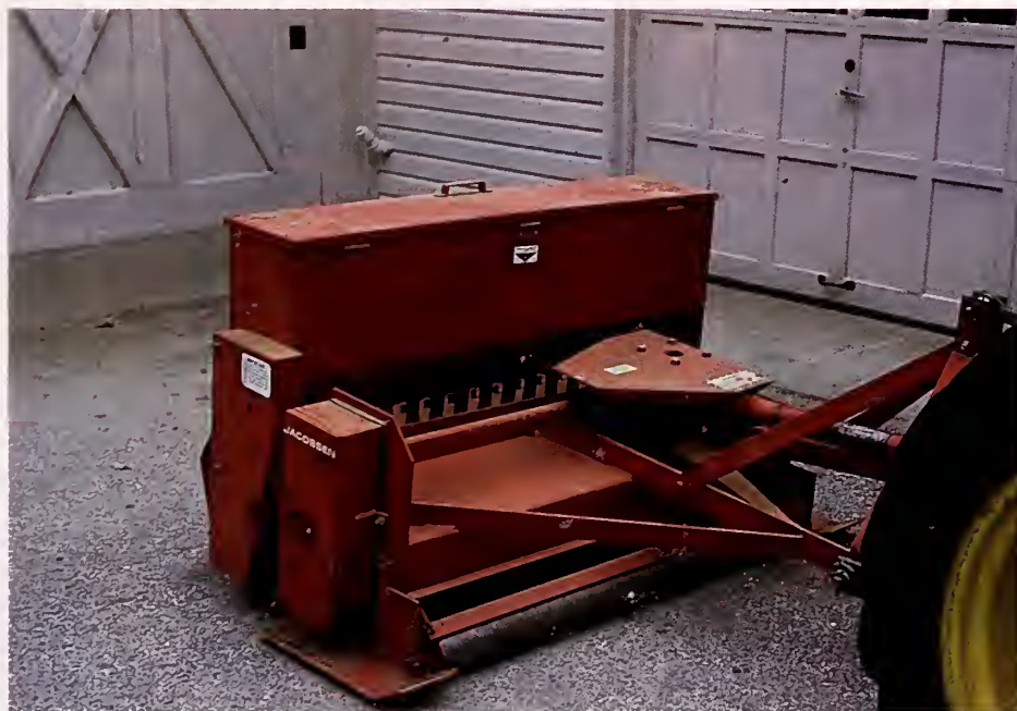
The seeder cuts a small trench in the ground and sows the seed within the trench.
