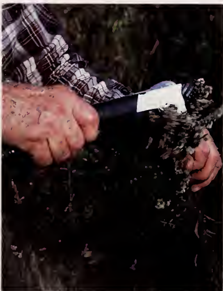
Bob DePuy assembled this vacuum for collecting seeds; it is powered by a 12-volt battery.
