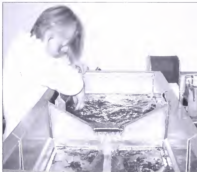
Figure 13-2: Sara Halwas using forced-air/froth flotation machine at the MUN lab.
