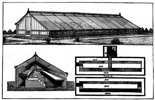
THREE-QUARTER SPAN GREENHOUSE FOR BOSE FORCING, ETC.
