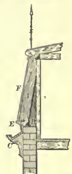
Section of Curb-roof. A, rafter, the foot of which projects over the plate B; C, cornice; F, bed-nook; F, slates or shingles.
