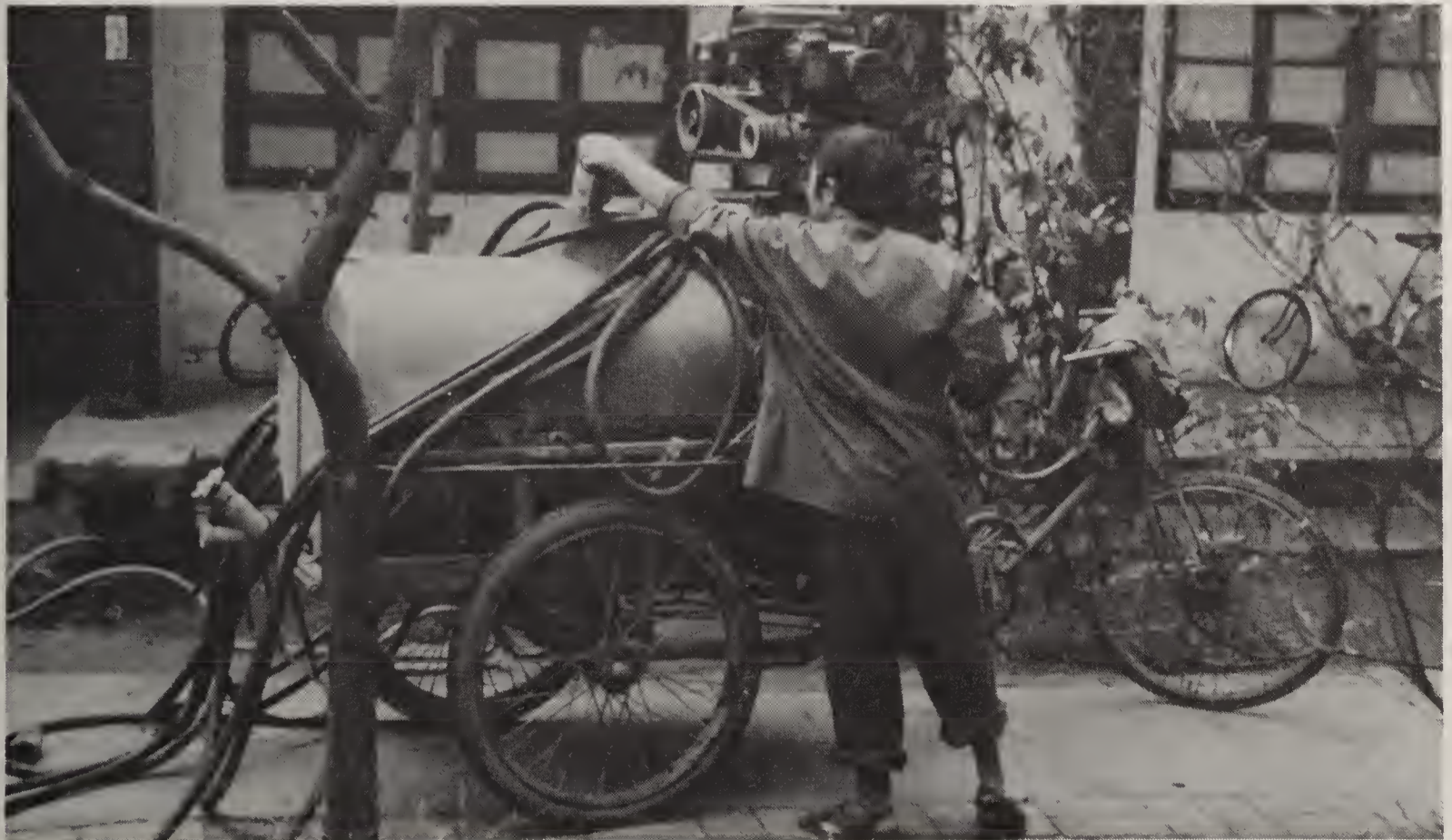
Bicycle-mounted pesticide sprayer
