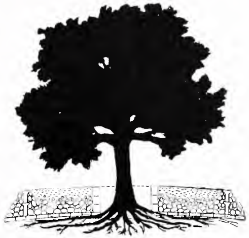
4. Cover whole area with rocks, then smaller stones, gravel, and thin straw layer to keep surface foot of topsoil from sifting in
