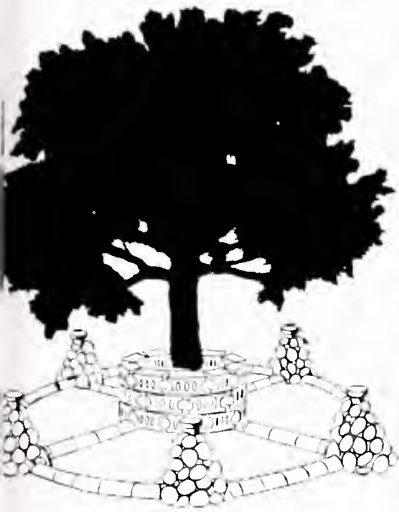
3. Stand 6" glazed tiles on spoke-rim junctions, with bell end up at fill level. Heap stones around to hold them upright
