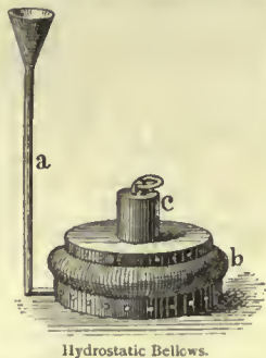
Hydrostatic Bellows. a, funnel-mouthed tube; b, box with flexible sides; c, weight.
