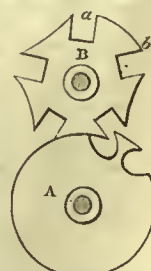
The Geneva Stop Movement, used in Swiss watches to limit the number of revolutions in winding up, the convexly curved part, a, of the wheel B serving as the stop.
