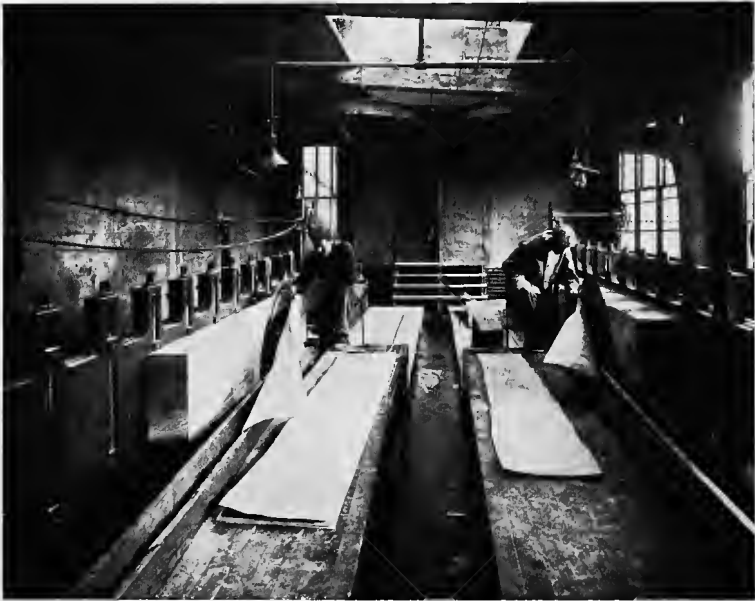
FIG. 20.—Making sawed veneers. Many of the finest veneers are made by this method.
