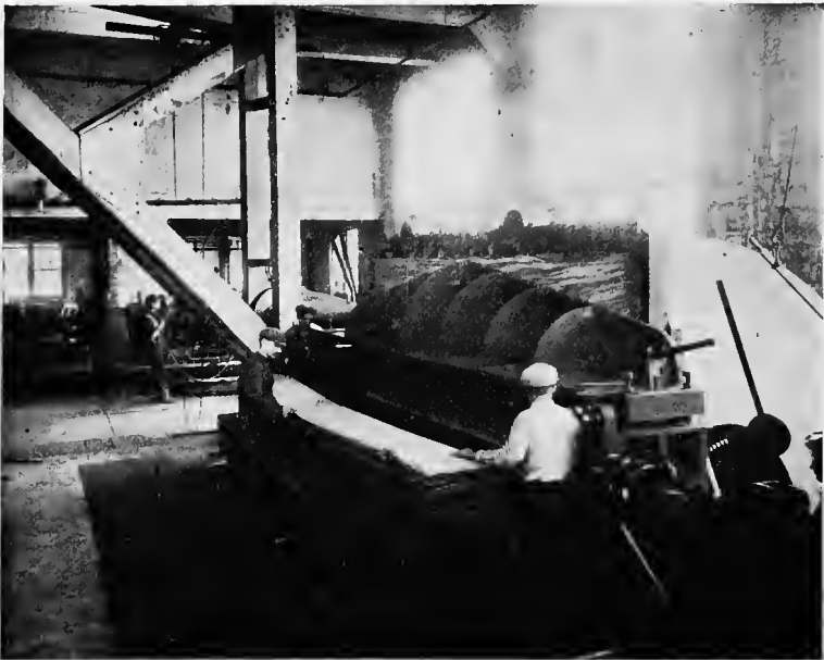
FIG. 19.—A veneer-slicing machine in operation, cutting Circassian walnut veneers. Note the veneer flitch fastened above. This is dropped vertically against a sharp knife. The men are engaged in piling the sliced veneers as they emerge at the base of the machine.
