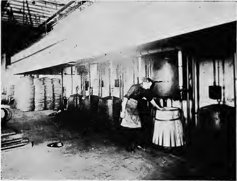
FIG. 41.—Method of heating the staves preliminary to placing them in a power windlass for final assembling.
