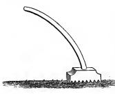
"Another method. The Botthammer is a wooden block (something of the size and shape of a denkee), having on its under face, channels or flutings, five or six deep lines, and it is fixed to a long bent helve or handle. In using it, a bundle of the dried Flax stalks is spread evenly upon the
