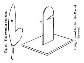
the breadth of this knife is important; when too narrow it easily causes the Flax to twist round it, and thereby tears a portion of the fibres. With this knife the Flax is repeatedly struck, parallel to the board (and close to the slit), with perpendicular blows, to scrape off its wooden asperities. The part which lies in the slit is continually changed by a motion of the left hand.
