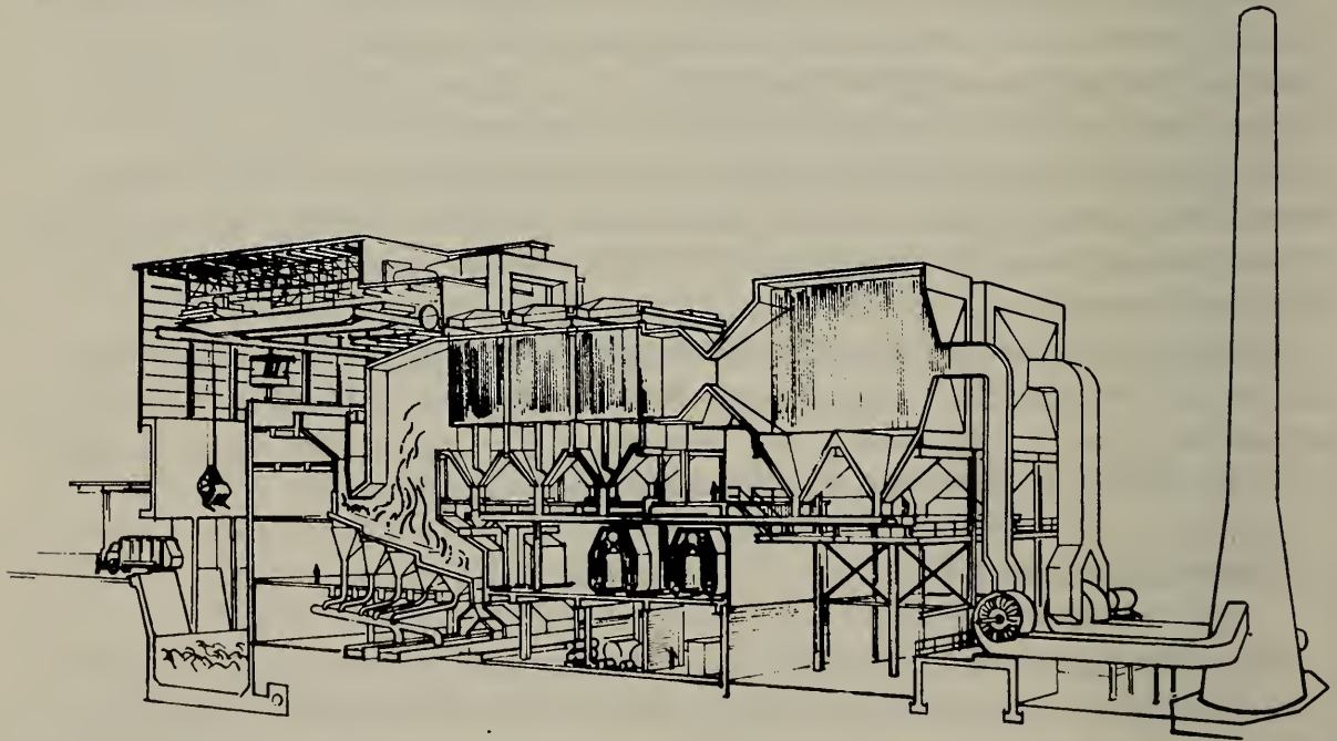
Fig. 2. Wheelabrator-Von Roll refuse-energy system.
