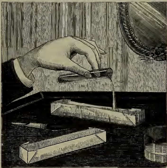
FIG. 3.—A PAPER BOX CLOSING UPON ITSELF WHEN WATER IS POURED INTO IT.
