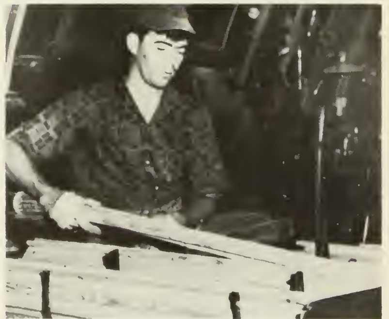
At a Whitefish woodworking plant, plywood peeler cores, normally waste material, are converted to snowfence laths.
