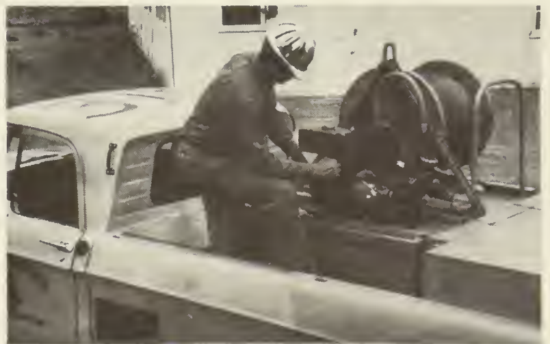
Four-wheel drive, heavy-duty pickup trucks, with 200-gallon water tanks, pumps, hose and nozzles, make excellent vehicles with which to get to and suppress wild fires quickly. The number painted on top of the cab identifies it to anyone who may be scouting the fire by airplane. This vehicle is located on the State Forester's Helena unit.
