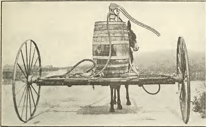
FIG. 21.—Ideal outfit for spraying cotton fields: Barrel pump with double lead of hose mounted on dismantled hayrake. (Original.)
