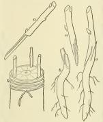
Fig. 2. Crown Grafting, Fig. 3. Tongue or Splice illustrated. Grafting.
