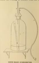
glass, parts with its latent heat, leaving the moisture it contained deposited on the ontside of the glass in the shape of dew. The reason why the temperature in nature never sinks lower than the dew point is plain. The air coming in contact with the cold earth and plants, parts with its moistnre. This changes from the vapour form into the liquid dew, which chauge results in freeing the latent heat contained in the vapor. Dew is
