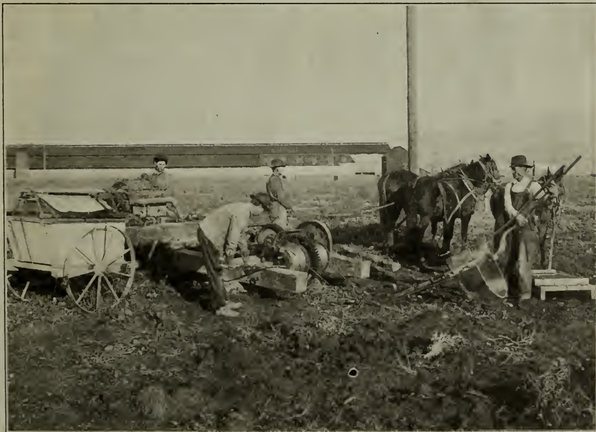
We find that this 40 H. P. gasoline engine is much more efficient than the old method of pulling the digger with horses. Four men handle the outfit.
