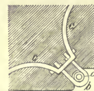
Collar and Clamp. a, hole for the pin of the leaf; b, clevis; c, c, anchor.
