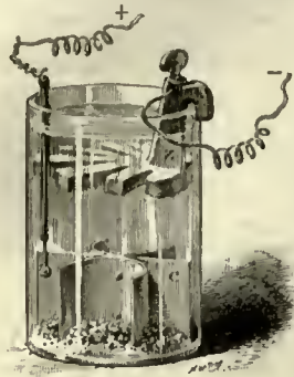
Gravity Cell. C, copper plate; Z, zinc plate.
