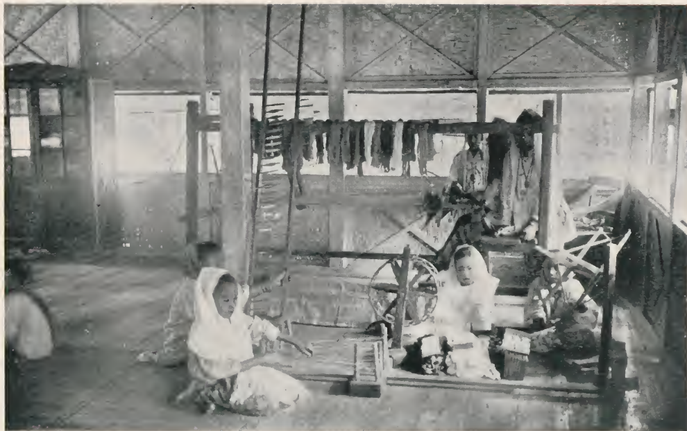
LAYING WARP THREADS FOR TRANSFERENCE TO LOOM, WINDING THREAD ON TO SPOOLS, AND WINDING THREAD FROM THE SKEIN.
