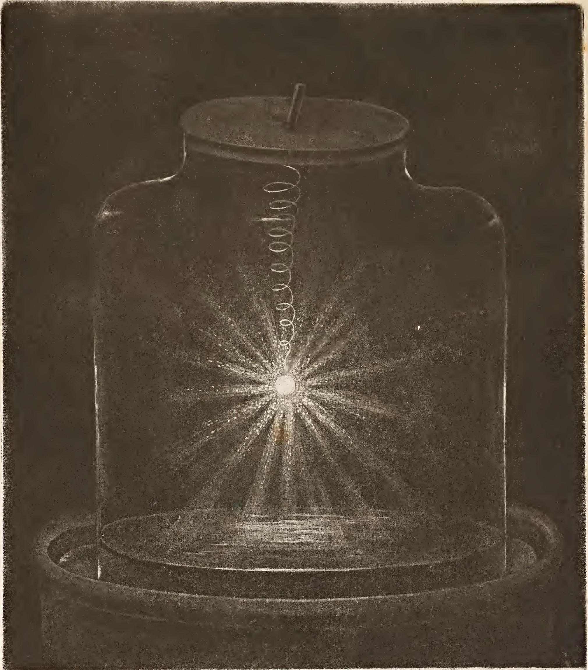
COMBUSTION OF A STEEL WIRE IN OXYGEN GAS.
