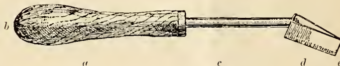
FIG. 2. Tool for incising Rubber Tree.
