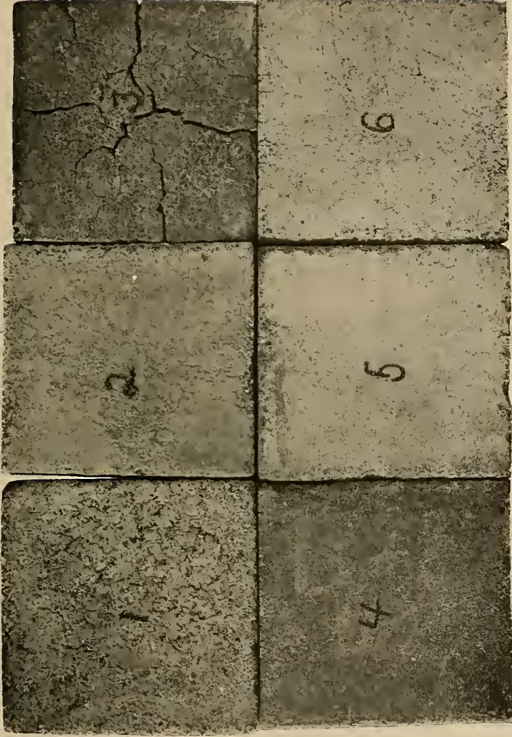
PLATE VII. SAND-LIME BRICKS MADE FROM PHILIPPINE RAW MATERIALS. HEATED TO 1,100° AND PLUNGED INTO WATER
