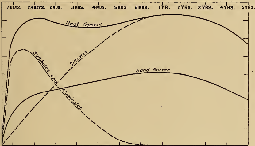
FIG. 23.—Typical curve of the tensile strength of Portland cement.
