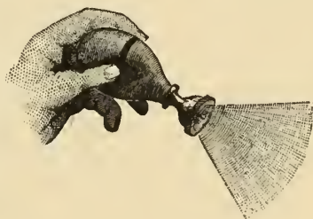
Improved Putty Bulb for Glazing Greenhouse Sash.
