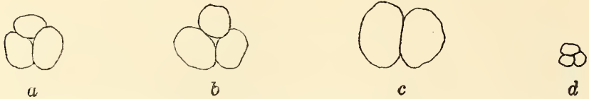
FIG. 1. Typical cross-sectional profiles of ropes tested. Actual size. a , rope made of Cordia cumingiana bast; b , rope made of Kleinhovia hospita bast; c , rope made of split bamboo ( Dendrocalamus merrillianus ); d , rope made of "F" grade abacá (machine laid).
