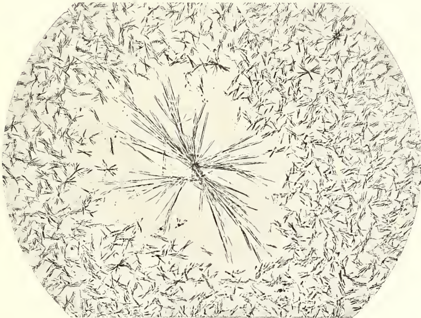
Fig. 2. Quick crystallization of the hydrochloride of the alkaloid.
