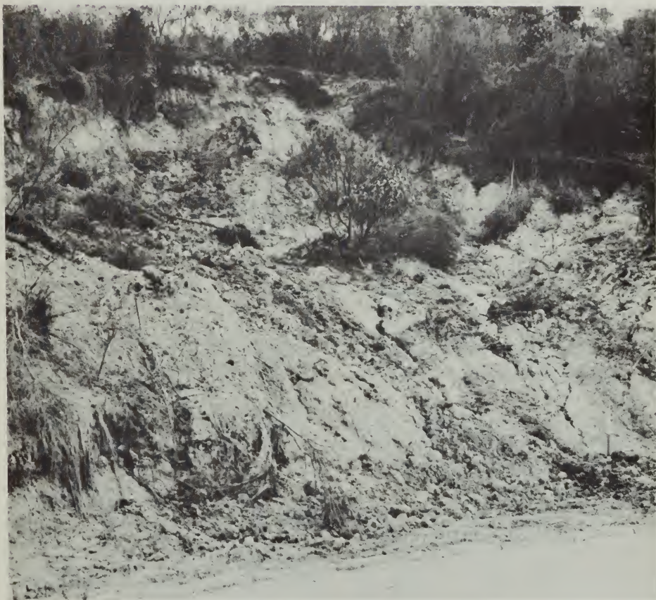
Plate 2. The area from which the slip came. Note that it is well vegetated. The slope is 25°, and the soil continues round the whole area, showing that it has been stable for a long time.
